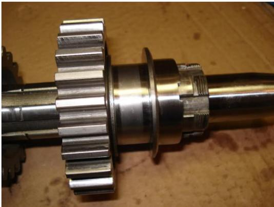
The first problem I have found is that the bushing is often too loose on the main shaft. So the first thing to do is press out the old bushing.
