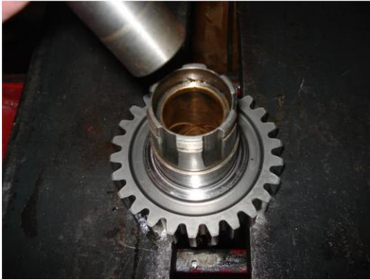
When the old bushing is out, I start by making a new one out of continuous cast bronze 660. Why making a new one? Often new bushings that came from different companies do not have enough material to clear everything, most of them, not to say all, are set at the factory to have minimal material to remove with a reamer, and often end up with many spots of material not removed.
