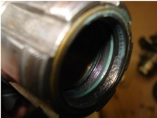
. When you are done with the gear, it is time to take care of the spacer, since the other main problem occur when some of the oil escape between the spacer and the shoulder of the gear, I always make a new type of spacer out of C1144 steel, with o ring groove inside so there is no way oil could escape.
