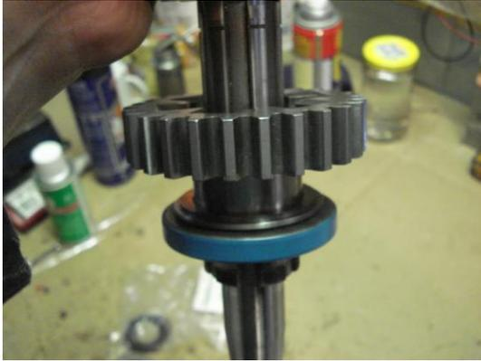
Here is the finished job with everything installed and ready to put the sprocket on. You could not see anything different from the outside, but this will definitely solve your leaking problem.
