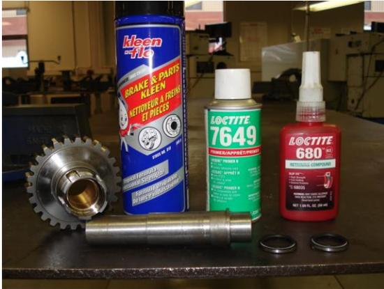
Since the outside seal will not receive too much oil, I simply put some Castrol synthetics grease between both seals, to make sure the seal outside get lubricate and cannot dry out.
