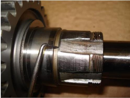
And the picture of the new spacer to accommodate the old gear.
