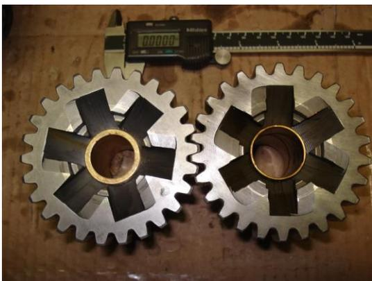
You will have to slightly polish the main shaft to get rid of small imperfection, or use a new shaft if it is too bad..., and then measure carefully so you could machine the bushing to achieve minimum clearance, in this case shaft measurement is .999 inch.
