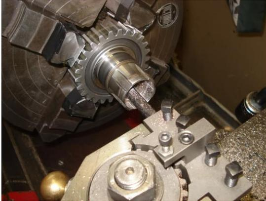
After the inside of the bushing is machined, I still continue modifying the end of the gear, here what I do, machining the recess a little bit deeper so I can put 2 seals in the end of the fourth gear instead of only one as OEM, the machining is done with either carbide or ceramic insert (much easier with a ceramic insert), the total depth required is 7/16 inch, instead of the 3/16 OEM, you can see the small oil groove inside the bushing not too deep but just enough to lubricate.
