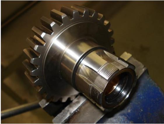
Note: that Andrews gear(late model) is now using an O ring seal on the shoulder of their gear, plus my spacer and includes one O ring on that run not far from their O ring, between end of spline and their O ring.
