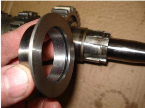
You could see the spacer with the o ring inside ready to be slip on the OEM gear, just put very small amount of grease around the o-ring to avoid scraping it.
