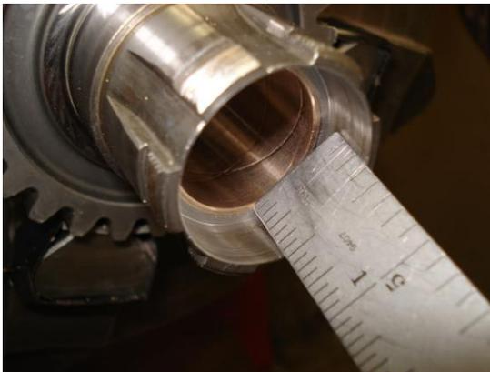
Ready to install the 2 new seals inside the end of the fourth gear: remember always clean /prime and put green Loctite on both the 2 small seals.
