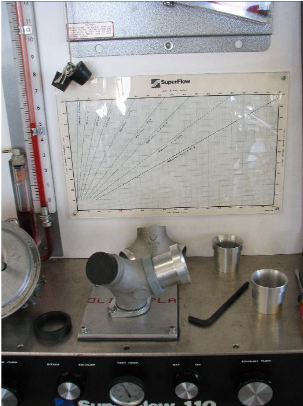
Figure 11 Carb Manifold Testing
