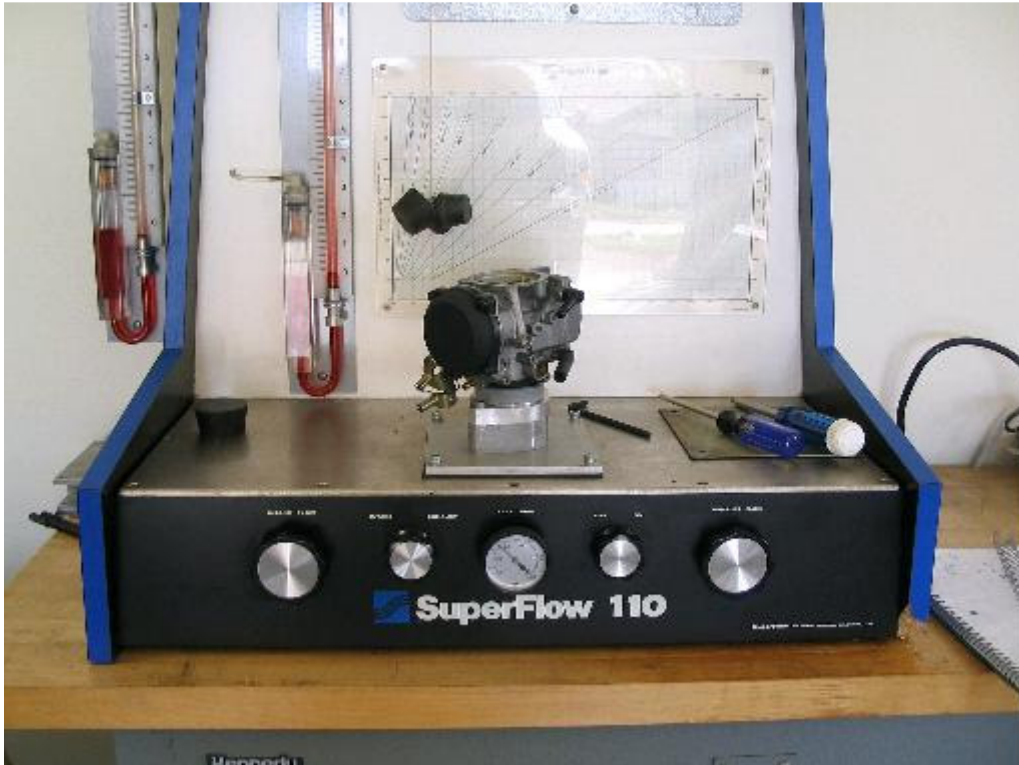
Here is a picture of the first flow test using a CV40 without air cleaner.
