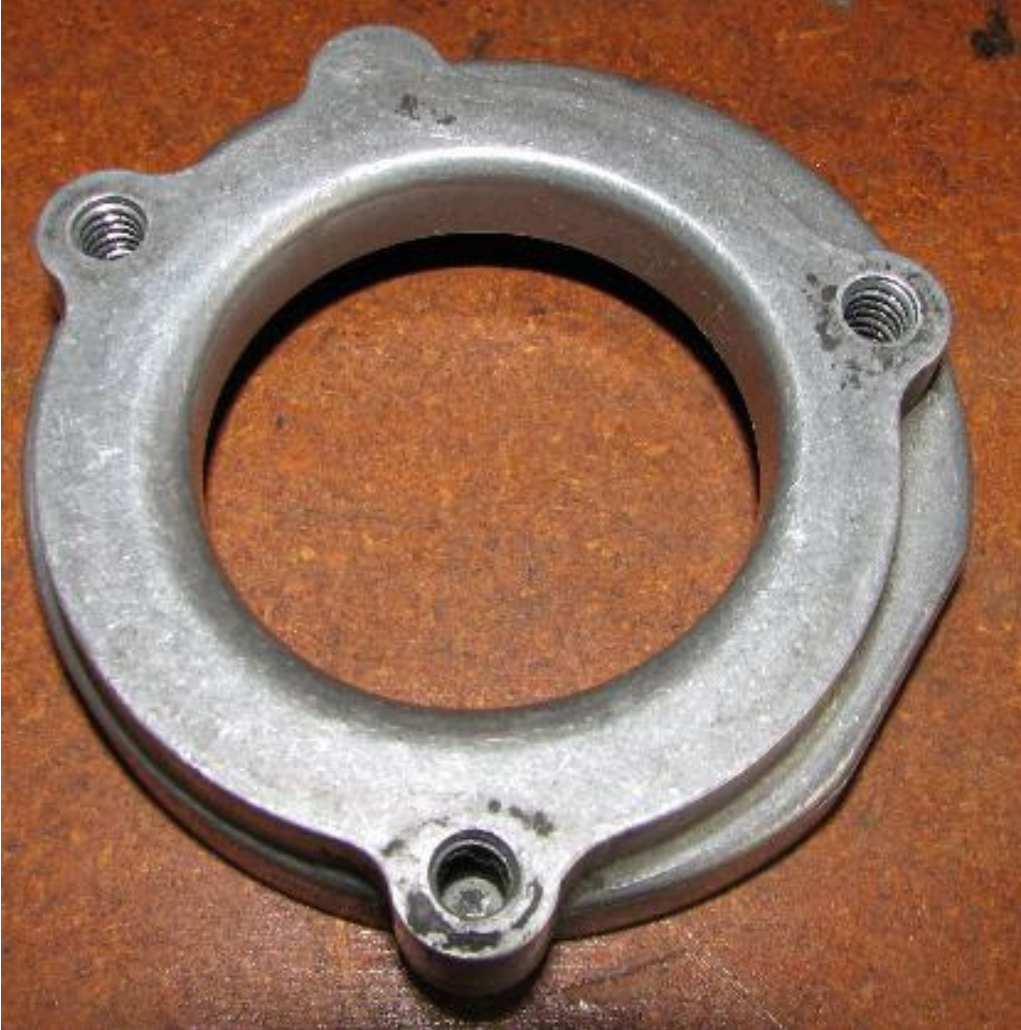
Figure 5 HSR to Backing Plate Adapter
