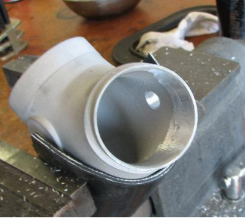
Figure 9 Blending the Taper
