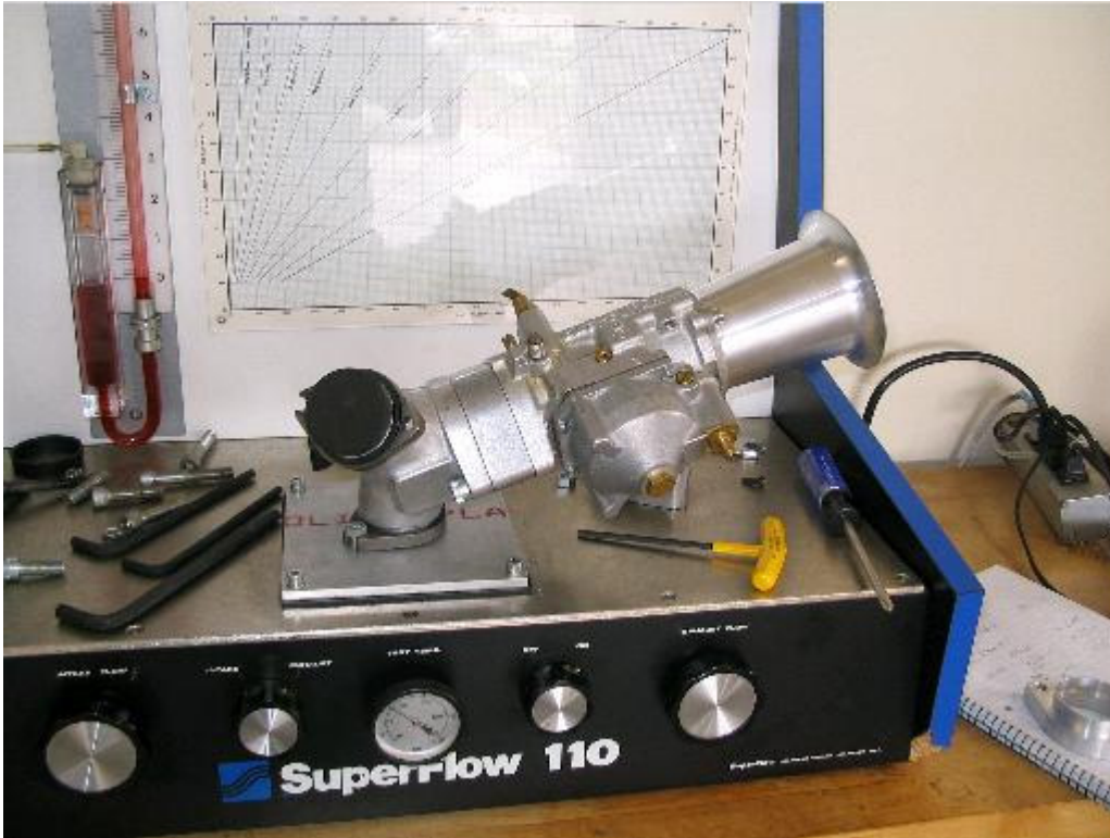
Super D with velocity stack on the intake manifold.
