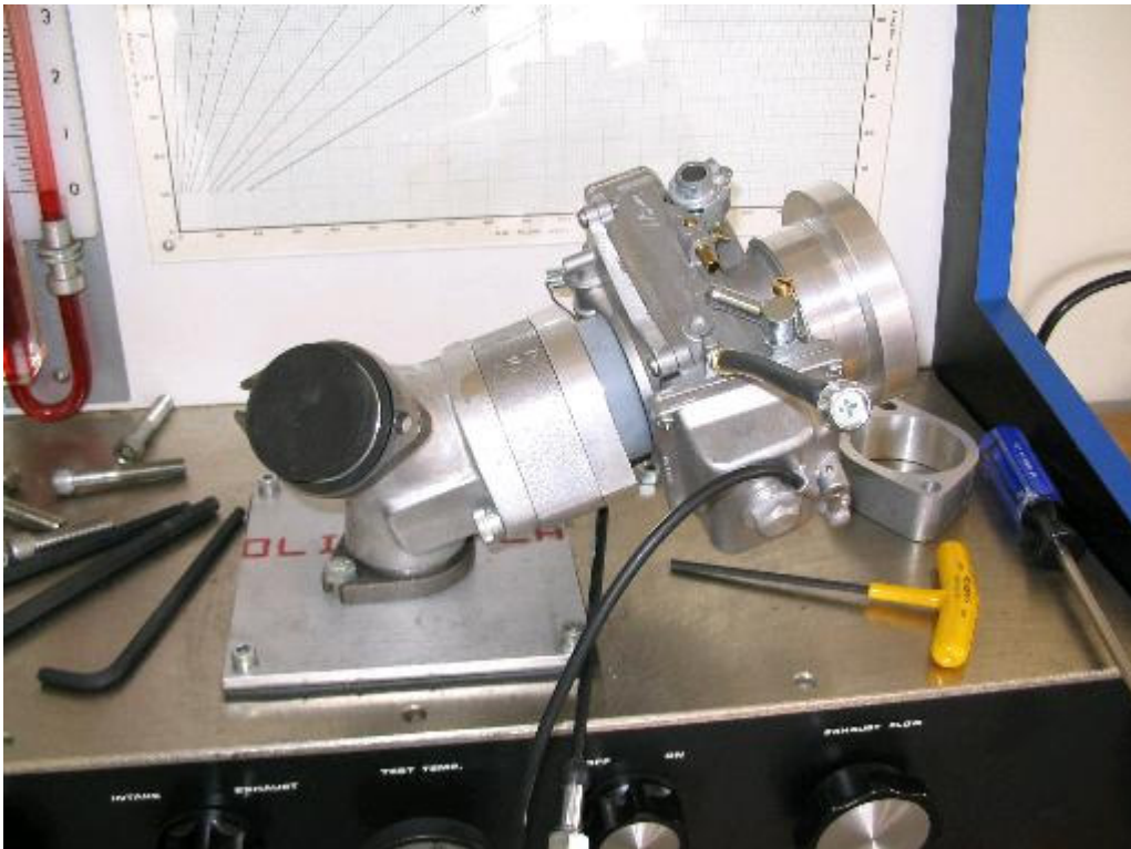
HSR45 in manifold with velocity stack.
