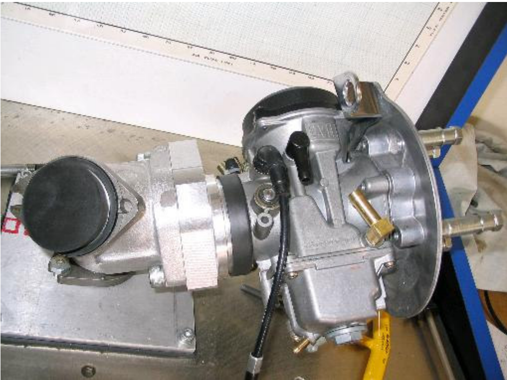
CV51 with dropped manifold adapter on super D manifold.
