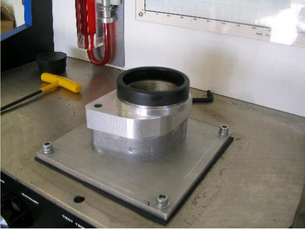
Dropped manifold on flow bench prior to fitting CV51.
