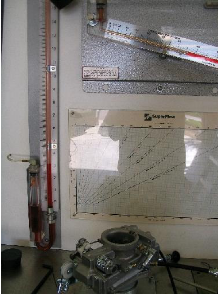
Here is an HSR48 with the Superflow running. Notice that the pressure is about 3 in of water vacuum and the flow is about 86%.
