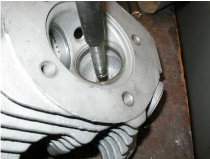
Pic 3 Driver in the guide ready for attack. Notice the Silver second step, I turned this down about .015" smaller than the OD of all the Shove guides
