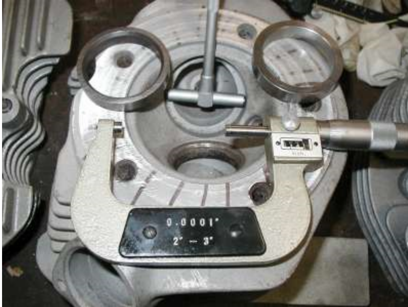
Pic 1 snap gauge in the hole and set, mic measured regular seat (left in the picture) oversize seat on right in pic.
